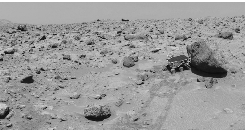
The Mars Pathfinder lander took this photo of its small rover, called Sojourner. Here, Sojourner is investigating a rock on Mars.
