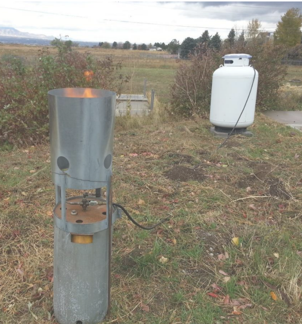
Example of a North America Weather Consultant manually operated Cloud Nuclei Generator, a cannister that projects silver iodide into the atmosphere. PHOTO COURTESY OF NAWC AND SANTA ANA WATERSHED PROJECT AUTHORITY
