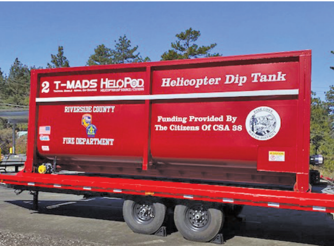
This is the portable HeloPod for firefighting to be stored at Pine Cove Water District. It can be transported to locations for helicopters to dip from. PHOTO BY BECKY SMITH
