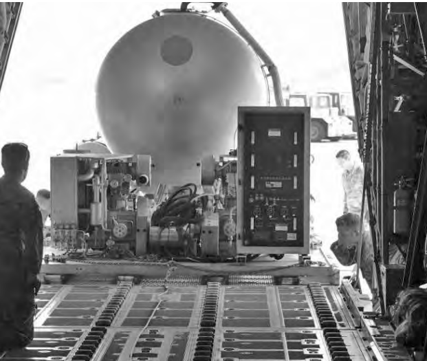
U.S. Air Force Loadmasters and Aerial Porters assigned to the 115th Airlift Squadron load a U.S. Forest Service Modular Airborne Firefighting System (MAFFS) inside a C-130J Super Hercules aircraft at Channel Islands Air National Guard Station, Port Hueneme, California, Sept. 7, 2022. MAFFS is a portable fire-retardant delivery system inserted into an aircraft, temporarily converting it into a firefighting airtanker that provides a critical “surge” capability to bolster wildfire suppression efforts when commercial airtankers are fully committed or not readily available.
